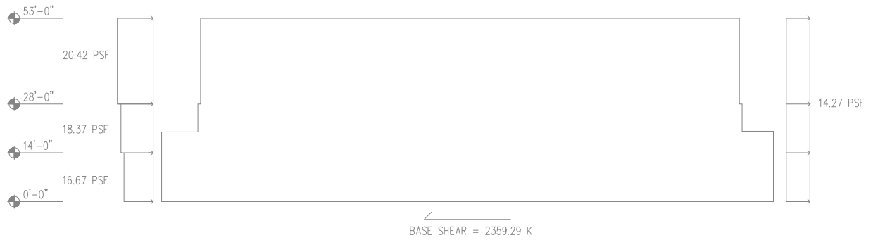
Figure 10 – North/South Wind Pressures
